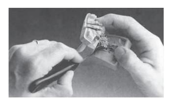
Castaldo White Label®, the less expensive of our two grades, has a high concentration of pure natural gum rubber, which makes it soft and pliable, qualities that the experienced mold-cutter values in their efforts to produce high-quality molds in the shortest reasonable time.
